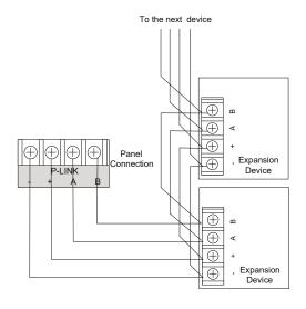
RA-6500 Class A Wiring Example Fig 2
